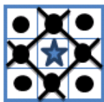
Figure 2. Two kinds of neighborhoods for a central cell: Von Neumann (x) and Moore (•)
